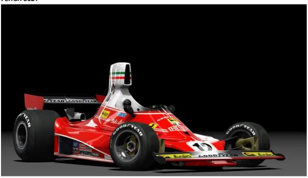
1975. The year of the 312 T, where the T stood for the transversal gearbox, in a 90-degree angle to the engine. This solution led to a compact engine and an improved weight distribution and a very fast and agile car, but also quite nervous and difficult to drive to the limit.
