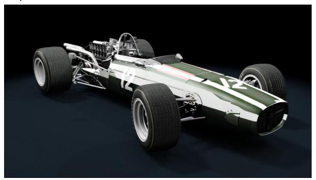
Derrick White was commissioned to design Cooper's very first monocoque chassis to house the Italian Maserati V12 engine. Dubbed the T81, the new 3-litre car was very conventional, perhaps with the exception of the front disc brakes, which were installed on the inside of the hub between the wishbones. Giulio Alfieri extensively reworked the almost ten year old engine, which produced a claimed 390 bhp.
