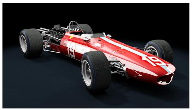
The McLaren M5A was a racing car constructed by Bruce McLaren Motor Racing, and was McLaren's first purpose-built Formula One car. Like its M4B predecessor, only one car of this type was ever built. The car was the first to use the BRM type 101 3.0 litre V12 engine, which produced 375 bhp.
