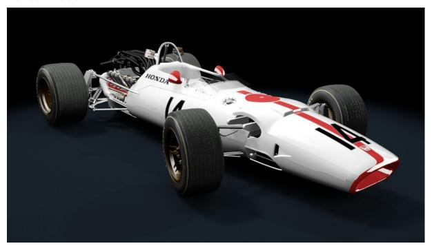
The Honda RA300 was a Formula One racing car produced by Honda Racing, and introduced halfway through the 1967 Formula One season. It retained the same V12 engine as the preceding RA273 car, but the chassis was designed by Lola's Eric Broadley and based on a previous Lola Indianapolis 500 car, the T90. This collaboration resulted in the machine being quickly dubbed the Hondola by the motorsports press.
