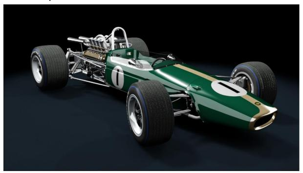
Following the trusty design principles a new single seater was designed for 1967; the BT23 for Formula 2 and the BT24 for Formula 1. The latter featured different suspension, brakes, wheels and gearbox to cope with the latest specification Repco engine, producing 350 bhp which was by no means impressive, but it did produce a very flat torque curve.
