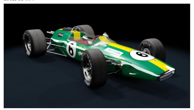
The Lotus 33's development was based on the earlier Lotus 25 model, taking the monocoque chassis design to new development heights. The 33 was almost identical to the 25, but had suspension designed around newer, wider tyres. The car was more rigid and was simpler to build than its predecessor. The last of the series, R14, was built with a 2-litre version of the Climax V8 for the 1966 World Championship season, pending the arrival of the Lotus 43.
