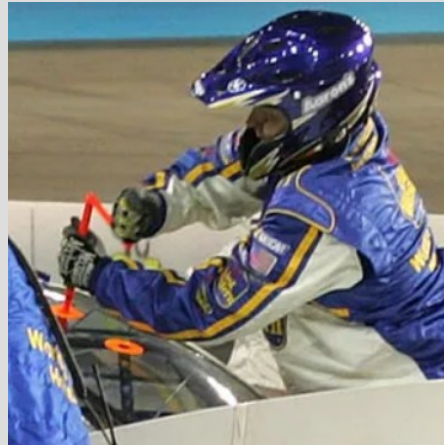
A NASCAR pit crew member making a right rear wedge adjustment during a pit stop.
