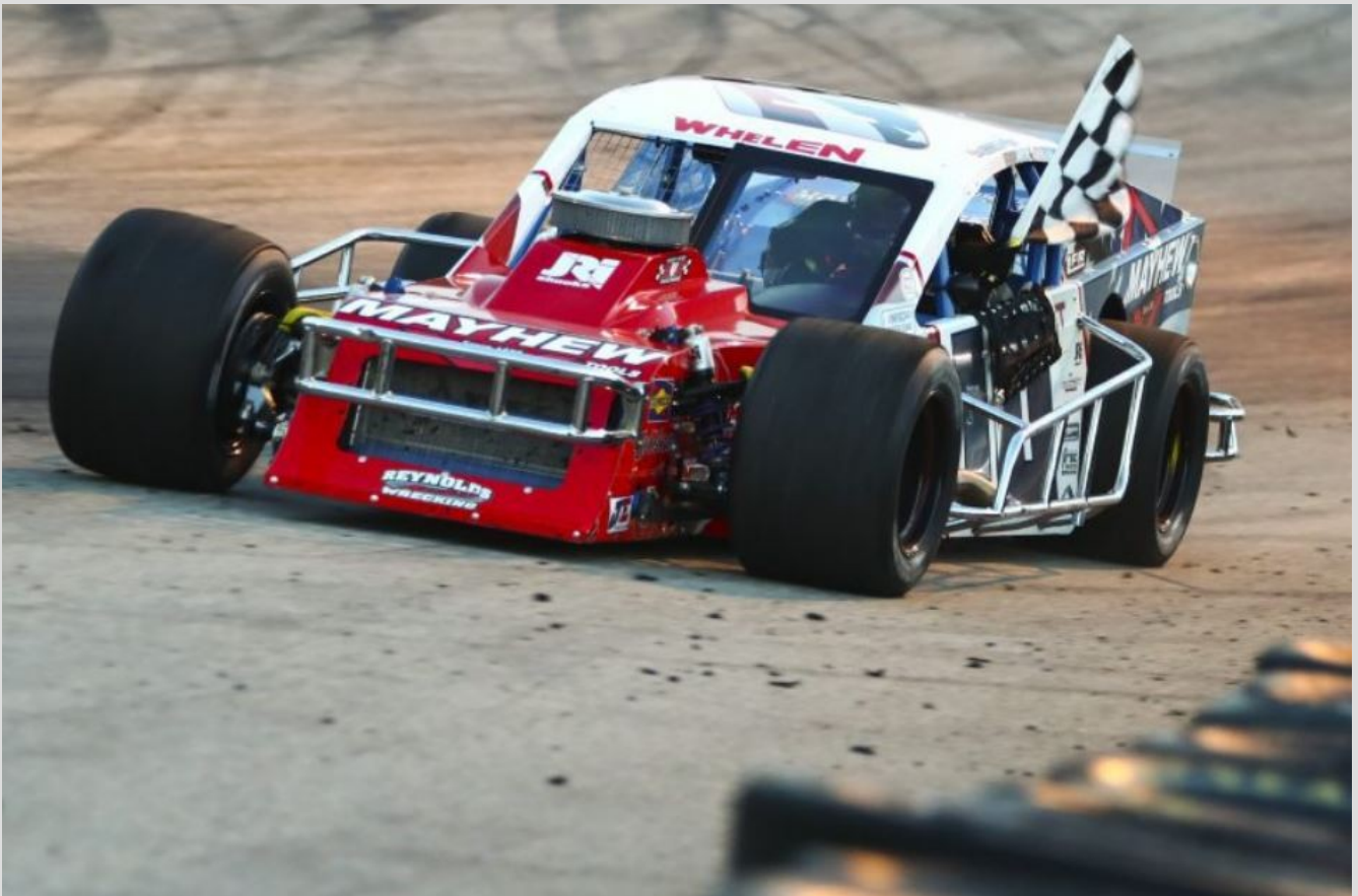
The open front wheels on Doug Coby's #10 Modified demonstrate circle track wheel camber.
