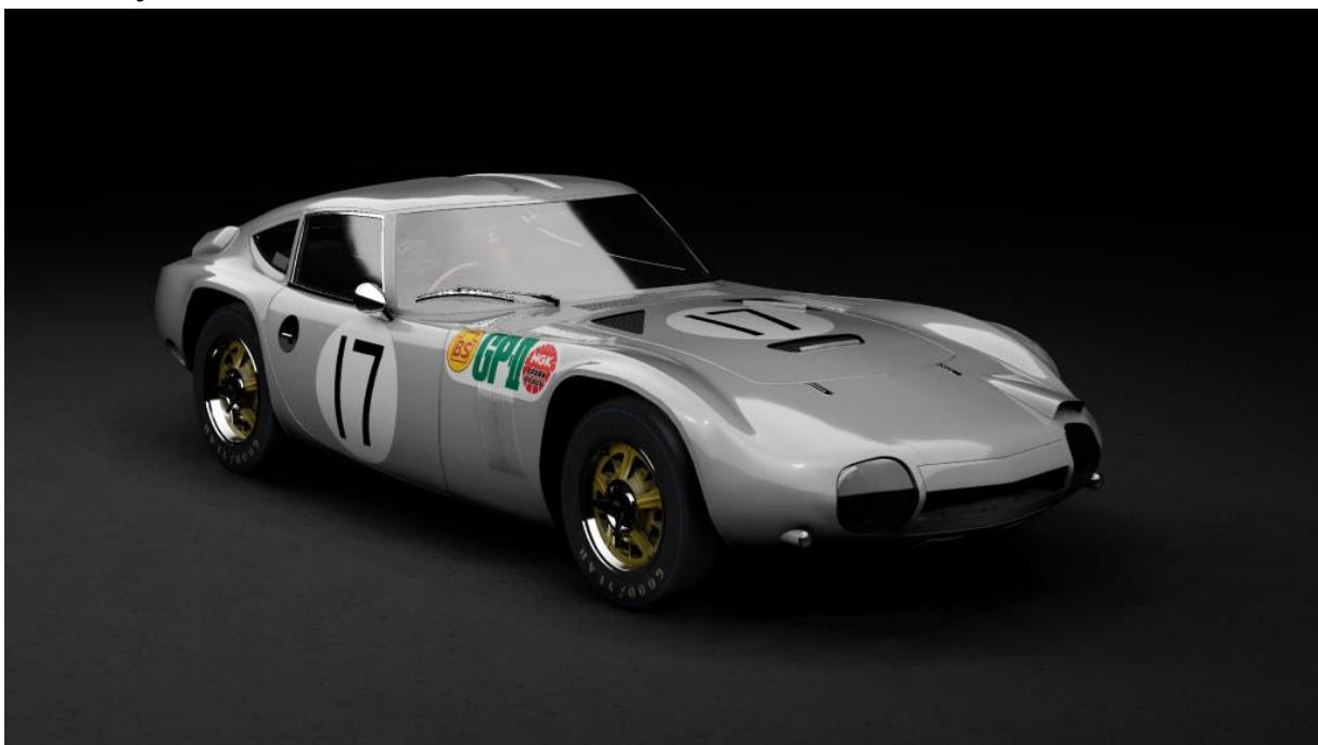
Toyota's pre-production 2000 GTs were assembled in two groups: the 280 A/I and 280 A/II, some of which came with aluminium bodies and others with steel. The most significant difference between the 280 A/I and 280 A/II was the latter's repositioned A-pillars which had been moved 40mm further forward to free up additional cockpit space.
