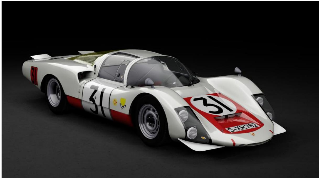
The story of the 906 LH begins with prototype chassis 906-016, which was completed on 28th November 1965. It deviated from the production 906s with a different engine mounting position that caused it to overheat - as discovered during restoration in the mid-2000s - and lower front and rear fenders with smaller and rounded-off cut-outs that reduced its frontal area from 1.325 m<sup>2</sup> to 1.318 m<sup>2</sup>.
